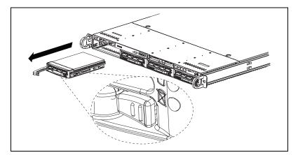
Figure B-25. Removing SCA Drive Tray
